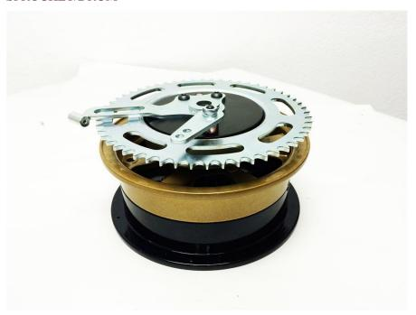
Your 215 Mini Bike is equipped with a lazer cut, precision welded, heavy duty Sprocket/Brake Drum to ensure smooth, reliable operation of the drivetrain.
