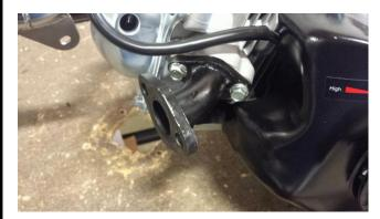
**Step 3** Installing the exhaust pipe
