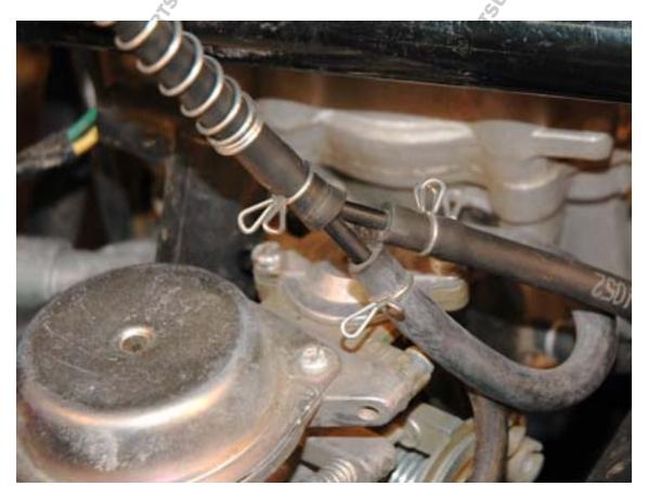
NOTE: Sometimes, the factory will plug the Y-connector into the Carburetor drain hose for shipment. If this is the case, disconnect the Y-connector, and then insert the Y-connector into the fuel tank's vacuum line. HAT SA.
