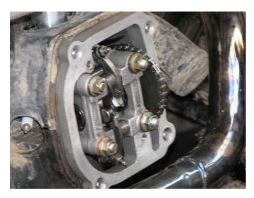
2. Rotate the camshaft until the big hole in the sprocket end points straight out of the top of the engine and the two smaller holes are lined up with the flat plane of the cylinder head. (Your camshaft may have lines instead of smaller holes, but they need to line up the same way). You can do this by rotating the variator in the CVT transmission counter clockwise by hand until the holes line up properly.
