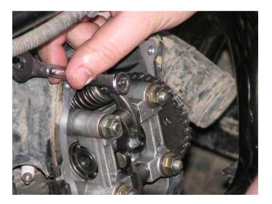
3. Use a wrench to loosed the retainer nut on the intake (top) valve.
