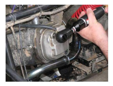
1. On some engine (kinroad) you may be able to adjust the valves directly on the engine. If not, remove the bolts holding the valve cover to the top of the engine.
